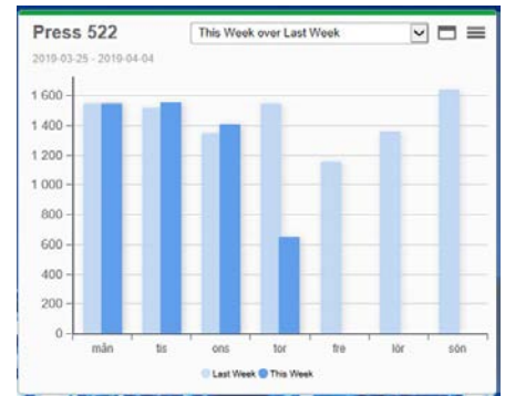
Kährs uses Schneider-Electric's Power Monitoring Expert software to monitor and evaluate energy consumption for the factory in Nybro at facility level and at machine level.
